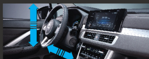
NEW STEERING WHEEL W/ TILT & TELESCOPIC ADJUSTMENT
